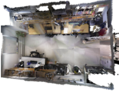
Fig. 2: A dense 3-D point cloud map that was built real-time (for offline use with our method) using an RGB-D sensor at 640x480 pixels resolution at a rate of 30 frames per second. This map was constructed as given in [2].
