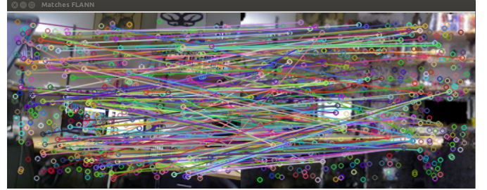
Fig. 4: Resulting SURF feature correspondences between real (left) and virtual (right) images (shown in Fig. 3b and Fig. 3a, respectively).
